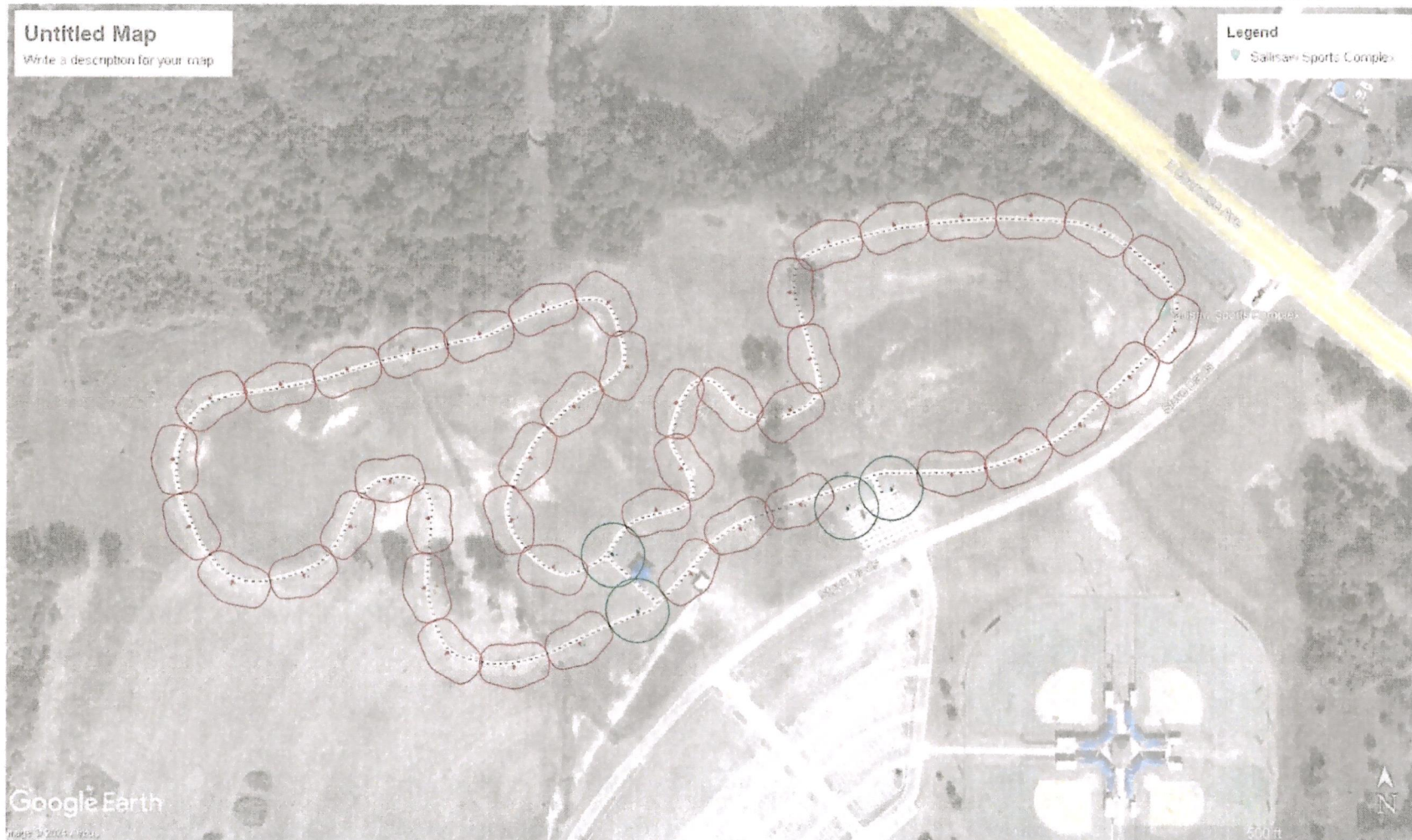
SALISAW SPORTS COMPLEX - TRAIL SOLAR LIGHTING - PHOTOMETRIC PLAN - 30W
